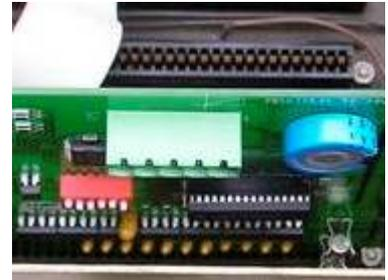
If a scoring system with standard APS is connected (Qubica, Steltronic, MaxS ...) dipswitch 6 must be in off position. To use the Qubica fast strike signal, the normally closed contact from the F-Box must be connected to pin 3 and 5 with dipswitch 6 in on position.
